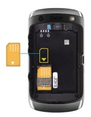
Slide the SIM card into the slot.
